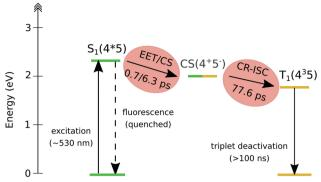
Scheme 2 Schematic representation of the decay pathway of dyad 3 upon photoexcitation of the Nile Red moiety.
