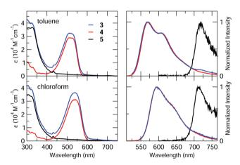
Fig. 3 Steady-state absorption (left) and normalized emission (right) spectra of the investigated compounds in toluene (top panels) and chloroform (bottom panels). Emission spectra of 3 were collected for excitation at  $\lambda$  = 515 nm in toluene and  $\lambda$  = 540 nm in chloroform
