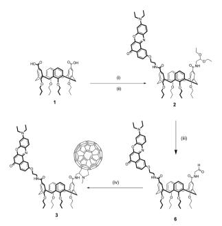
Scheme 1 Synthesis of Nile Red- $C_{60}$  calix[4]arene 3: (i) (COCl)<sub>2</sub>, DMF, DCM, 5 h, r.t., quantitative; (ii) 2,2-diethoxyethanamine, NR-NH<sub>2</sub>, DIPEA, DCM, 12 h, r.t., 47%; (iii) HCl (1M), dioxane, 4 h, r.t., 77%; (iv) C<sub>60</sub>, sarcosine, toluene, reflux, 3 h, 23%.
