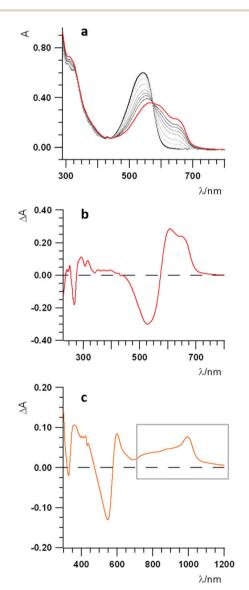
Fig. 5 (a) UV-Vis-NIR spectra of 0.6 mM dyad 3 in 0.08 M TBAH/DCM solution; working electrode, Pt gauze; temperature = 0 °C. Spectra of the pristine compound (black line) and one-electron reduced species (red line). (b) Difference spectrum of the reduced state (red trace; spectrum of the pristine compound subtracted). (c) UV-Vis-NIR difference spectrum of the oxidized state of dyad 3 0.6 mM in 0.08 M TBAH/DCM solution; working electrode, Pt gauze; temperature = 0 °C.
