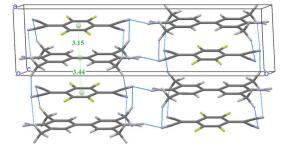
Fig. 5 Crystal structure of TMB-TCNQF4 at 100 K. The network of hydrogen bonds and the intermolecular distances (in Å) along the stack are also shown
