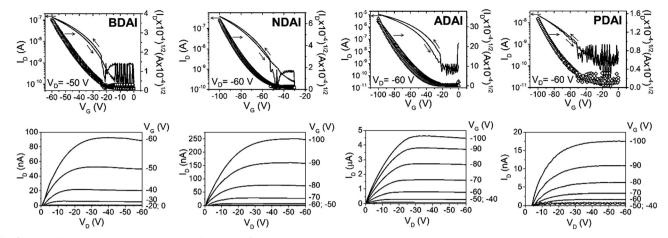
Fig. 2 Transfer and output characteristics of thin-film OFETs.
