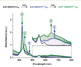
Fig. 5 UV-Vis absorption spectra of neutral (black), cation (blue) and dication (green) species of ZnP-2EDOTV-C60 (1), in dichloromethane solution, generated upon successive additions of FeCl<sub>3</sub>.
