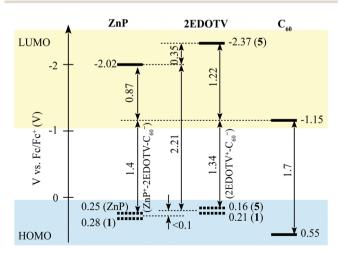
Fig. 2 Relative energy positions of HOMO and LUMO levels of the chromophores constituting the Zn-2EDOTV-C<sub>60</sub> triad.
