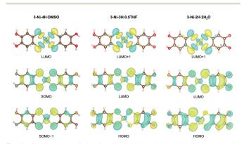
Fig. 4 Distributions of the frontier orbitals of the nickel complexes in 3-Ni-4H·DMSO, 3-Ni-3H·0.5THF, and 3-Ni-2H·2H₂O. These figures were visualized by VESTA.<sup>60</sup>
