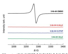
Fig. 3 ESR spectra of 3-Ni-4H-DMSO, 3-Ni-3H-0.5H<sub>2</sub>O, 3-Ni-3H-0.5THF, and 3-Ni-2H·2H<sub>2</sub>O. The black, red, blue, and green solid lines indicate the spectra of 3-Ni-4H-DMSO, 3-Ni-3H-0.5H<sub>2</sub>O, 3-Ni-3H-0.5THF, and 3-Ni-2H·2H<sub>2</sub>O, respectively. The ESR signals derived from the electron spins were not observed in the crystals except for 3-Ni-4H-DMSO
