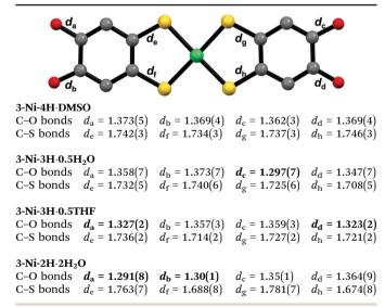
$d_{\rm d}$  = 1.323(2) Å for 3-Ni-3H-0.5THF; Table 1, Fig. S7 and S8, ESI†); their lengths are intermediate between the lengths of single-bond C–O ( $\sim$ 1.37 Å, *cf.* non-deprotonated 3-Ni-4H-DMSO) and double-bond C–O ( $\sim$ 1.23 Å, *cf.* nickel *o*-benzoquinonedithiolene complex<sup>42</sup>). These results indicate that these hydroxy groups with
