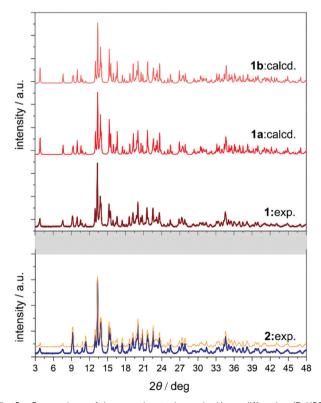
Fig. 2 Comparison of the experimental powder X-ray diffraction (P-XRD) pattern measured for **1** with the patterns for **1a** and **1b** calculated based on structural models obtained from the SC-XRD method (top), together with the experimental P-XRD pattern gathered for **2** which was compared with the pattern (orange line) obtained from the LeBail fitting procedure performed using EXPO 2014 software (bottom).
