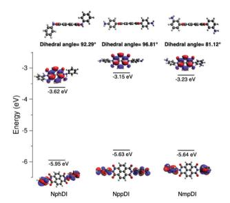
Fig. 8 Energy scheme and the HOMO and LUMO isosurfaces for NphDI, NppDI, and NmpDI (left to right).
