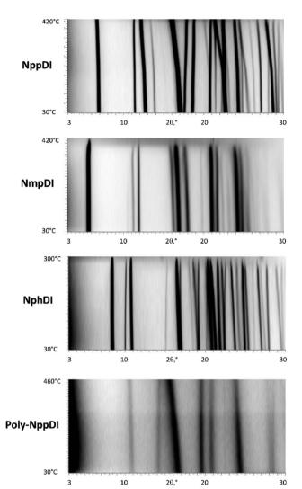
Fig. 5 Variable temperature XRD scans ( $2\theta$  in the  $3-30^{\circ}$  range), from RT (bottom) to 420, 420, 300, and 460 °C, respectively.
