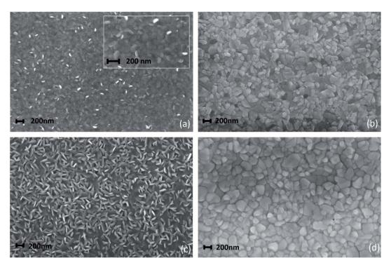
Fig. 6 SEM images collected on (a)  $Pbl_2$  deposited on an ITO/PTAA substrate using a deposition time of 15 minutes and (b) the converted MAPbl<sub>3</sub> after 30 minutes of MAI deposition. (c)  $Pbl_2$  deposited for 30 minutes and (d) the resultant MAPbl<sub>3</sub> after 60 minutes of MAI deposition.
