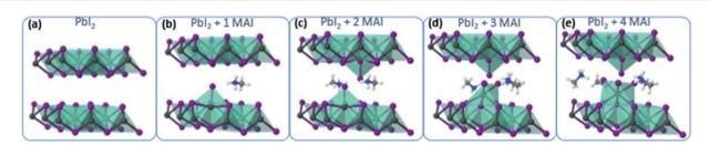
Fig. 4 DFT calculations of MAI intercalation within  $Pbl_2$  layers. (a) Ideal  $Pbl_2$  structure and intercalation of (b) 1 MAI molecule, (c) 2 MAI molecules, (d) 3 MAI molecules and (e) 4 MAI molecules within the layers of the  $Pbl_2$  structure.
