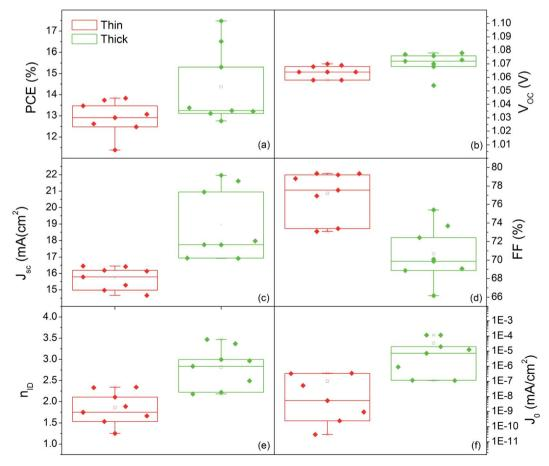
Fig. 10 Box plot of (a) efficiency (PCE), (b) open circuit voltage ( $V_{oc}$ ), (c) short circuit current ( $J_{sc}$ ), (d) fill factor (FF), (e) ideality factor ( $n_{iD}$ ) and (f) reverse saturation current ( $J_0$ ) from the electrical characterization of all the prepared devices with 80 nm thick and 150 nm thick MAPbI<sub>3</sub> active layers.
