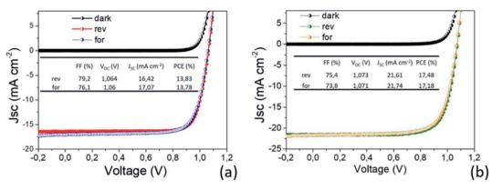
Fig. 9 /-V characterization of the best prepared devices with (a) 80 nm and (b) 150 nm MAPbl<sub>3</sub> active layers. The AVT moves from 32.8% to 20%.
