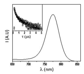
Fig. 8 Emission spectrum (main, exc = 405 nm) and corresponding lifetime decay (inset, exc = 405 nm; em: 750 nm) of MAPbl<sub>3</sub> thin film on glass.
