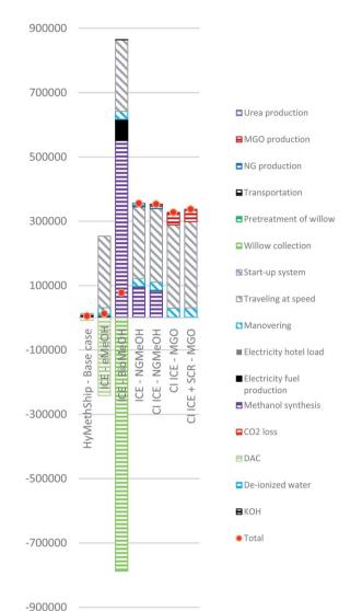
Fig. 5 Process contribution to climate change (GWP100) for all cases. Unit kg CO<sub>2</sub> equivalents. Presented per round trip between Gothenburg and Kiel on a RoPax vessel.
