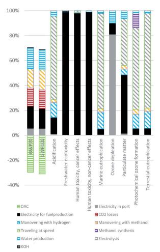
Fig. 3 The contribution to each impact category presented per process in the life cycle of the HyMethShip concept as described in Section 2 and scenario A in Fig. 2. Combustion processes for propulsion include travelling at speed, maneuvering with hydrogen, and maneuvering with methanol. Electricity for fuel production includes electricity production from offshore wind power used in direct air capture, methanol synthesis, and electrolysis.
