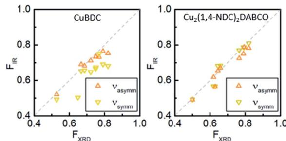
Fig. 3 Correlation of degree of orientation  $F$  obtained from XRD and FTIR spectroscopy in transmission for CuBDC and Cu<sub>2</sub>(1,4-NDC)<sub>2</sub>-DABCO films for  $\nu_{\text{symm}}(\text{COO}^-)$  and  $\nu_{\text{asymm}}(\text{COO}^-)$  bands.
