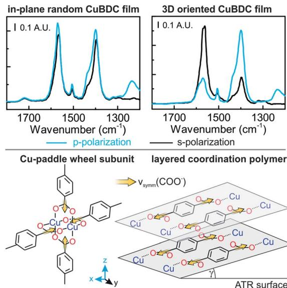
Fig. 8 (Top) Polarization-dependent ATR spectra of CuBDC prepared from random and aligned  $\text{Cu}(\text{OH})_2$ . Background spectrum = blank Si ATR crystal. (Bottom) Cu-paddle wheel subunit found in 2D MOFs and BDC linker alignment in a layered coordination polymer. The transition dipole moment of the  $\nu_{\text{sym}}(\text{COO}^-)$  bands are indicated by yellow arrows.
