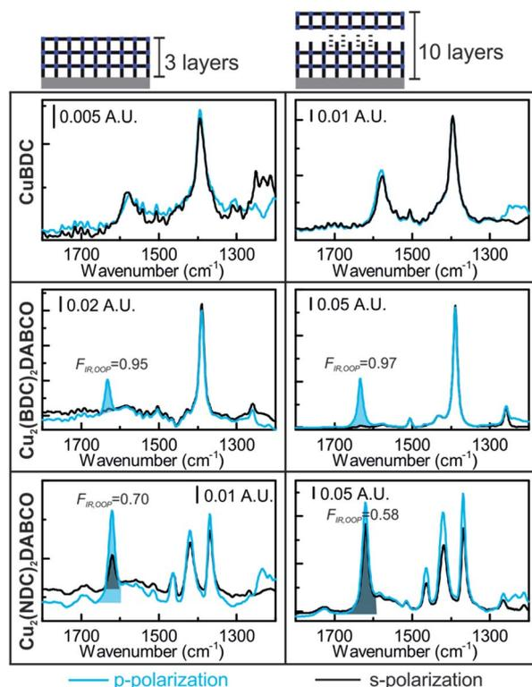
Fig. 6 Polarization-dependent ATR-IR spectra of MOF films prepared with the layer-by-layer method with 3 and 10 layers. The  $\nu_{\text{asymm}}(\text{COO}^-)$  band of both 3D MOFs,  $\text{Cu}_2(\text{BDC})_2\text{-DABCO}$  and  $\text{Cu}_2(1,4\text{-NDC})_2\text{-DABCO}$ , shows strong polarization dependence, which allows to calculate the degree of out-of-plane orientation from the band areas. Background = blank Si ATR crystal.
