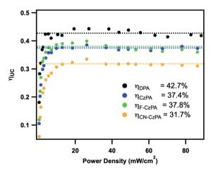
Fig. 5 Upconversion quantum efficiencies measured for 0.25 mM acceptors/annihilators sensitized by  $\rm Zr(^{Mes}PDP^{Ph})_2$  (OD<sub>514 nm</sub> = 0.2) in deaerated THF solutions as a function of excitation power density at 514.5 nm.
