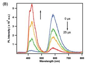
Fig. 3 Transient absorption difference spectra (A), and time-resolved photoluminescence spectra (B) of  $Zr(^{Mes}PDP^{Ph})_2$  (OD<sub>514 nm</sub> = 0.4) and 0.25 mM DPA in deaerated THF at several delay times following 514 nm pulsed laser excitation (~2 mJ per pulse) with delay times indicated.
