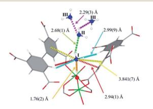
Fig. 19 Binding sites for  $ND_3$  molecules adsorbed within MFM-300(Al) determined by *in situ* NPD studies. Reprinted with permission from ref. 110. Copyright (2018) John Wiley & Sons.
