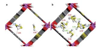
Fig. 10 Illustrative arrangements of H<sub>2</sub>S in the pores of MIL-53-TDC generated from the GCMC simulations at (a)  $0.5 \text{ mmol g}^{-1}$  and (b) 18.5 mmol  $g^{-1}$ . The distances are reported in Å. (Al, pink; O, red; S, yellow; C, grey; H, white). Reprinted (adapted) with permission from ref. 69. Published (2019) by The Royal Society of Chemistry.
