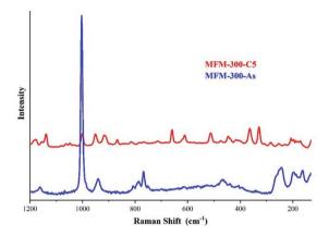
Fig. 11 Raman spectra of MFM-300(Sc) after 5 cycles of  $H_2S$  (red) and as synthesised (blue). The peaks observed in the  $350-520~{\rm cm}^{-1}$  region are associated to the S–S stretching vibrations modes of several polysulphides with various chain lengths. Reprinted with permission from ref. 70. Copyright (2020) American Chemical Society.
