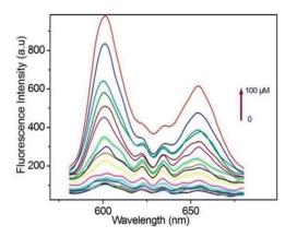
Fig. 14 Fluorescence spectra of porphyrin ligand (10  $\mu$ M) in BBS butter (pH = 7.40, 20 mM) after titration with HS $^-$  from 0–100  $\mu$ M,  $\lambda_{ex}=419$ . Reprinted with permission from ref. 94. Copyright (2014) American Chemical Society.
