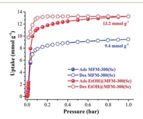
Fig. 4  $SO_2$  adsorption isotherm of scandium-based MFM-300 (blue isotherm) and after confinement of 2.8% EtOH (red isotherm). Reprinted with permission from ref. 37c. Published (2019) by The Royal Society of Chemistry.
