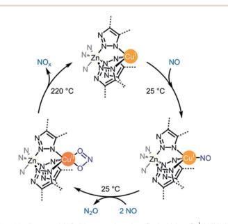
Fig. 26 Proposed NO Disproportionation Cycle Using  $Cu^{I}$ -MFU-4l. During the thermal decomposition of Cu-MFU-4l(NO $_{2}$ ), NO is the major NO $_{x}$  species detected. Reprinted with permission from ref. 126. Copyright (2021) American Chemical Society.
