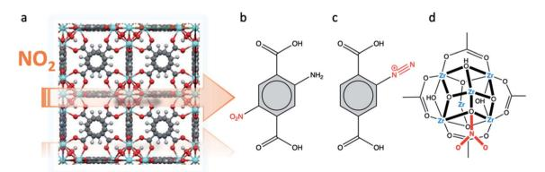
Fig. 23 (a) Structure of UiO-66 analogues. Post functionalization of phenyl ring modifications upon  $NO_2$  sorption: (b) nitration of the phenyl ring, (c) diazonium ion formation. (d) Nitration of the bridging hydroxyl group at the SBU. Reprinted (adapted) with permission from ref. 123. Copyright (2016) John Wiley & Sons.
