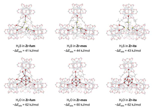
Fig. 7 DFT-calculated structures of  $H_2S$  binding in Zr-fum, Zr-mes, and Zr-ita with calculated energies of adsorption ( $-\Delta E_{ads}$ ) indicated. The DFT-calculated structures and energies of  $H_2O$  adsorption in all three MOFs are included for comparison. Gray, white, red, yellow, and pale blue spheres correspond to carbon, hydrogen, oxygen, sulfur, and zirconium, respectively.
