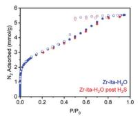
Fig. 5 77 K  $N_2$  adsorption isotherms of activated Zr-fum- $H_2O$ , Zr-mes- $H_2O$ , and Zr-ita- $H_2O$  before (blue) and after treatment with  $H_2S$  at 25 °C (red). After  $H_2S$  adsorption, the MOFs were regenerated at 100 °C under vacuum (<10  $\mu$ bar) for 48 h.
