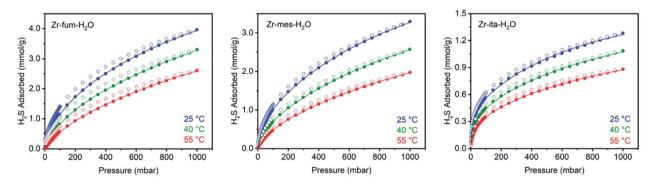
Fig. 3 H<sub>2</sub>S adsorption (closed circles) and desorption (open circles) isotherms at 25 °C (blue), 40 °C (green), and 55 °C (red) of activated Zr-fum-H<sub>2</sub>O, Zr-mes-H<sub>2</sub>O, and Zr-ita-H<sub>2</sub>O. Solid lines represent fits of the adsorption data to a Langmuir-Freundlich model. A data point was considered equilibrated after <0.01% pressure change occurred over a 45 s interval.
