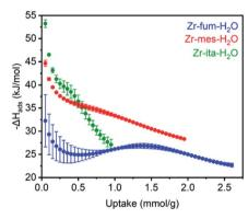
Fig. 4 Differential enthalpies of adsorption ( $-\Delta H_{ads}$ ) for H<sub>2</sub>S as a function of uptake for activated Zr-fum-H<sub>2</sub>O (blue), Zr-mes-H<sub>2</sub>O (red), and Zr-ita-H<sub>2</sub>O (green), as determined using the Clausius-Clapeyron equation (eqn (1)) and Langmuir-Freundlich fits in Fig. 3. A data point was considered equilibrated after <0.01% pressure change occurred over a 45 s interval.
