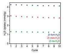
Fig. 6 Cycling capacities for  $H_2S$  adsorption (1 bar, 30 °C) in Zr-fum- $H_2O$ , Zr-mes- $H_2O$ , and Zr-ita- $H_2O$ . The samples were regenerated at 100 °C under high vacuum (<10  $\mu$ bar) between cycles.
