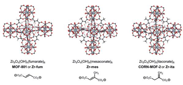
Fig. 1 Density functional theory-calculated ideal structures of known and new sustainably-derived metal-organic frameworks prepared from fumaric, mesaconic, and itaconic acid as part of this work. Gray, white, red, and pale blue spheres correspond to carbon, hydrogen, oxygen, and zirconium, respectively.
