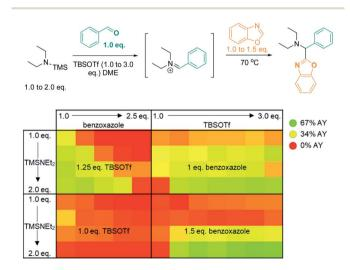
Scheme 5 Optimization via high-throughput screening: influence of 3 variables (benzoxazole, TBSOTf, and Et<sub>2</sub>NTMS loading) on product yield. AY = assay yield, as determined by calibrated UPLC analysis (210 nm), using biphenyl as internal standard.
