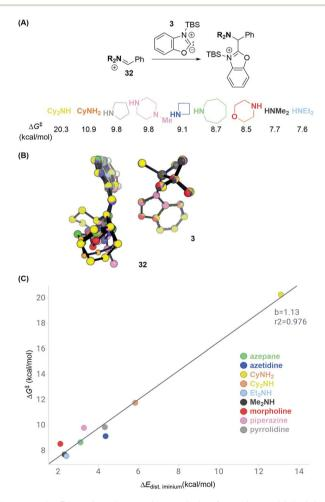
Scheme 12 Distortion–interaction analysis of reactions with iminium electrophiles. (A) Transition state energies  $\Delta G^{\ddagger}$  for series of iminium electrophiles. (B) Overlay of transition state structures. (C) Distortion energies  $\Delta E_{\rm dist}$  versus  $\Delta G^{\ddagger}$  of C–C bond formation. See ESI† for details of computational methods. M06-2X/def2TZVPP/SMD(ether)//M06-2X/6-31G(d)/SMD(ether).
