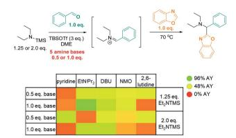
**Scheme 6** High throughput screen: base optimization. AY = assay yield, as determined by calibrated UPLC analysis (210 nm), using biphenyl as internal standard.
