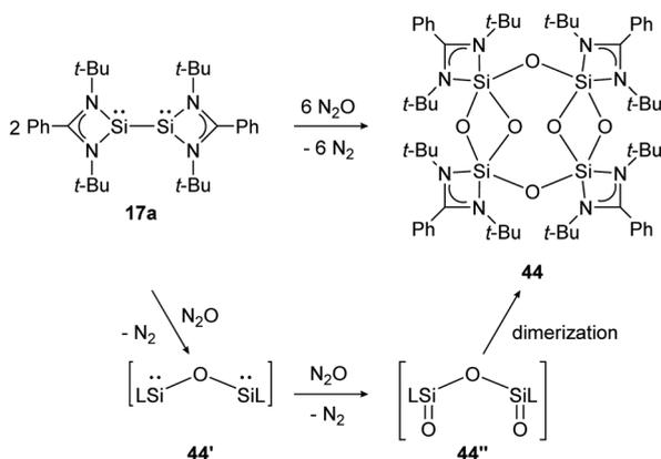
Scheme 19 Reactivity of bissilylene **17a** with  $\text{N}_2\text{O}$ .<sup>130</sup>
