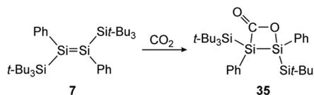
Scheme 10 [2 + 2] cycloaddition of  $CO_2$  to supersilyl substituted disilene **7**.<sup>85</sup>
