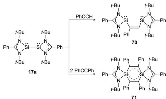
Scheme 32 Cycloaddition reactions of bissilylene **17a** with phenylacetylene and diphenylacetylene.<sup>140</sup>
