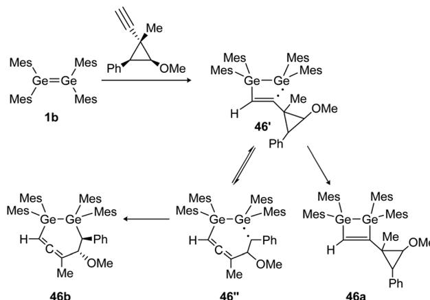
Scheme 21 Reaction of tetramesilyldigermene with a cyclopropyl alkyne. Mes = 2,4,6-trimethylphenyl.<sup>134</sup>
