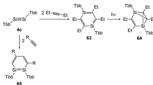
Scheme 30 Cycloaddition reactions of disilyne **4c** with mono and disubstituted acetylene derivatives  $\text{R} = \text{H}, \text{Ph}$ .<sup>47,49</sup>
