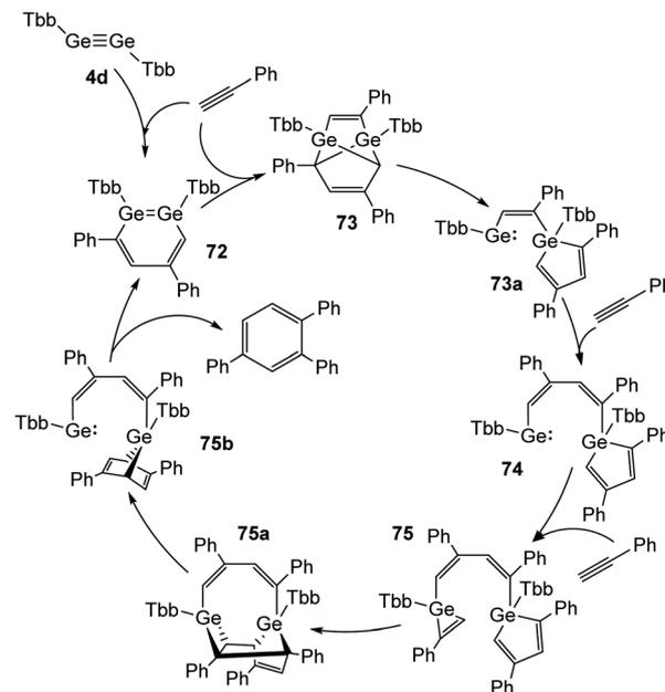
Scheme 33 Full catalytic cycle for the cyclotrimerization of phenylacetylene using digermene **4d**.<sup>16</sup>
