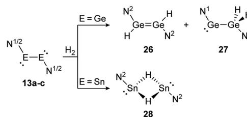
Scheme 6 Reactivity of bisgermylenes **13a** and **13b** and bisstannylene **13c** with H<sub>2</sub>. N<sup>1</sup> = N(Ar<sup>1</sup>) (SiMe<sub>3</sub>) (Ar<sup>1</sup> = 2,6-(CHPh<sub>2</sub>)<sub>2</sub>-4-MeC<sub>6</sub>H<sub>2</sub>), N<sup>2</sup> = N(Ar<sup>2</sup>) (Si-*i*-Pr<sub>3</sub>) (Ar<sup>2</sup> = 2,6-(CHPh<sub>2</sub>)<sub>2</sub>-4-*i*-PrC<sub>6</sub>H<sub>2</sub>).<sup>61,92,93</sup>
