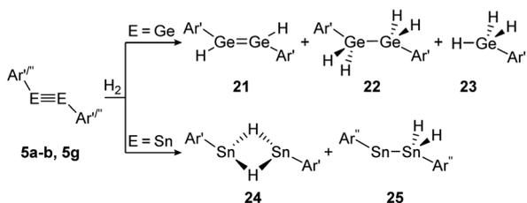
Scheme 5 Reactivity of digermynes **5a** (Ar' = C<sub>6</sub>H<sub>3</sub>-2,6-(C<sub>6</sub>H<sub>3</sub>-2,6-*i*-Pr<sub>2</sub>)<sub>2</sub>) and distannynes **5b** and **5g** (Ar'' = C<sub>6</sub>H-2,6-(C<sub>6</sub>H<sub>2</sub>-2,4,6-*i*-Pr<sub>3</sub>)<sub>2</sub>-3,5-*i*-Pr<sub>2</sub>) with H<sub>2</sub>.<sup>110–112</sup>
