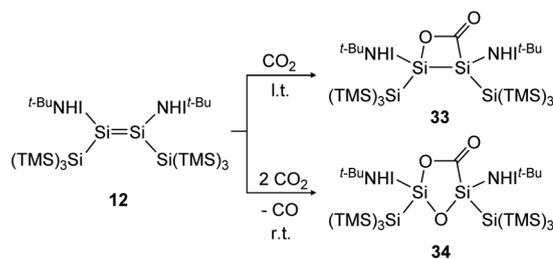
Scheme 9 Activation of  $CO_2$  by iminodisilene **12** at l.t. =  $-78^\circ C$  or r.t. = room temperature. TMS =  $SiMe_3$ .<sup>91</sup>
