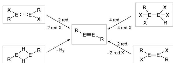
**Scheme 2** Possible synthesis routes for the isolation of dimetallenes. E = Si, Ge, Sn, Pb; R = stabilizing ligand; X = halogen; red. = reductive agent. Note: Hydrogen elimination route (bottom left) is only known for E = Sn, Pb.
