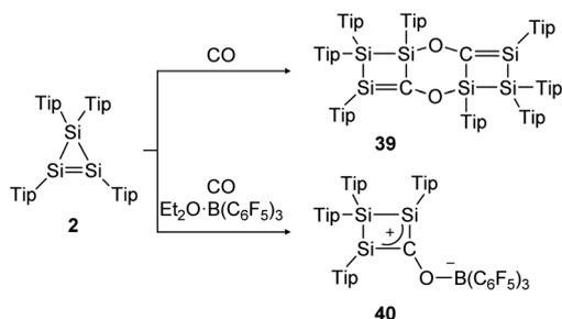
Scheme 14 Reactivity of cyclotrisilene **2** with CO and additional Et<sub>2</sub>O·B(C<sub>6</sub>F<sub>5</sub>)<sub>3</sub>. Tip = 2,4,6-triisopropylphenyl.<sup>124,125</sup>
