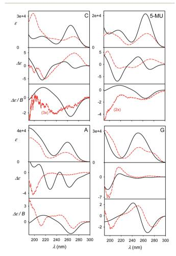
Fig. 6 Calculated (black solid) and experimental (red dashed) spectra of four nucleosides, obtained as an average of 200 MD geometries (B3LYP/6-311++G\*\*/CPCM calculation, no explicit waters).
