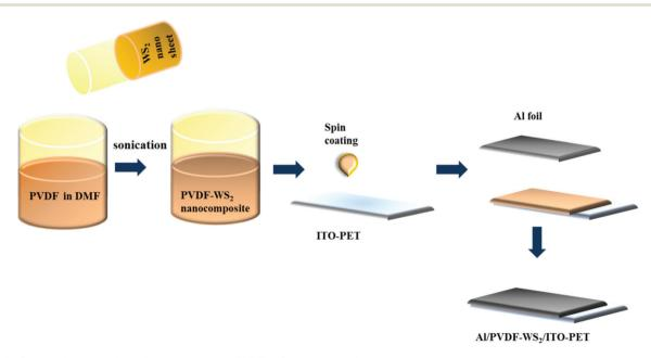
Scheme 1 Schematic of the fabrication process of the PVDF-WS2 composed piezoelectric nanocomposite device.
