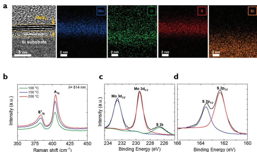
**Fig. 2** (a) High-resolution cross-sectional TEM image of MoS<sub>2</sub> multilayer on Si substrate and EDS mapping images of molybdenum, oxygen, sulfur, and silicon elements. (b) Raman spectrum of MoS<sub>2</sub> film synthesized using AP-PECVD with different processing temperature (100, 150, and 200 °C). (c, d) XPS spectra of the MoS<sub>2</sub> film obtained by AP-PECVD.
