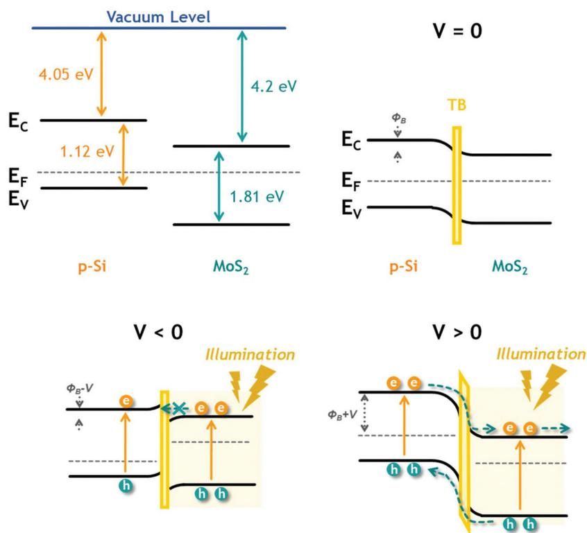
Fig. 4 Energy-band diagrams of the MoS<sub>2</sub>/Si photodetector before forming heterojunction, at equilibrium ( $V = 0$ ), forward bias ( $V < 0$ ) and reverse bias ( $V > 0$ ) under illumination, respectively.
