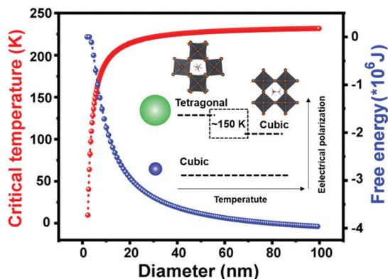
Fig. 8 Critical temperature and Gibbs free energy versus particle diameter for  $\text{MAPbBr}_3$  PQDs based on Ginzburg–Landau–Devonshire theory. Reproduced with permission from ref. 144. Copyright 2019, American Chemical Society.
