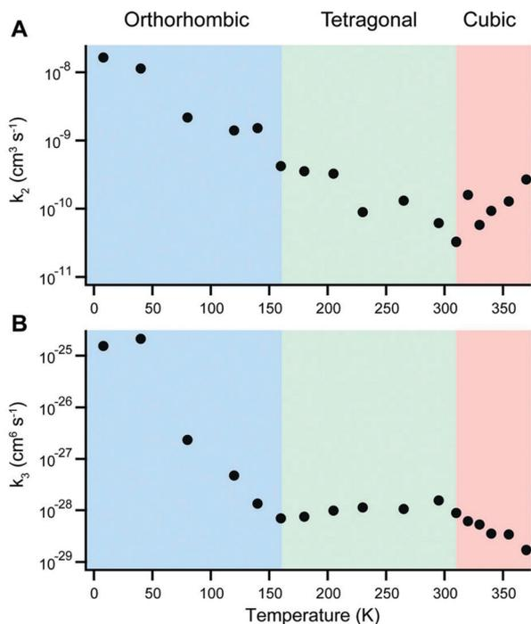
Fig. 14 Temperature dependence of (A) bimolecular and (B) Auger recombination rates for MAPbI<sub>3</sub>. Reproduced with permission from ref. 11. Copyright 2015, Wiley.
