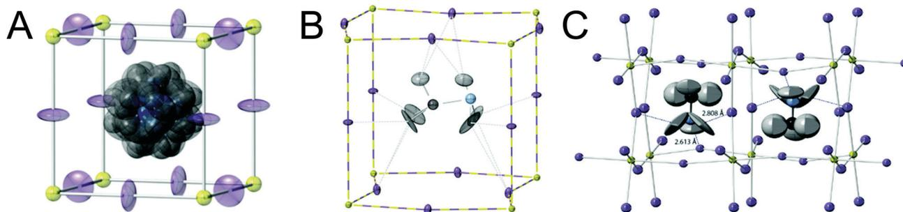
Fig. 5 Depictions of MA<sup>+</sup> cation orientations in the (A) cubic phase with ADP ellipsoids at 50% probability, (B) one orientation of the tetragonal phase with ADP ellipsoids at 50% probability, and (C) orthorhombic phase with ADP ellipsoids at 90% probability of MAPbI<sub>3</sub>, as determined by powder neutron diffraction experiments. Adapted with permission from ref. 43. Copyright 2015, Royal Society of Chemistry.
