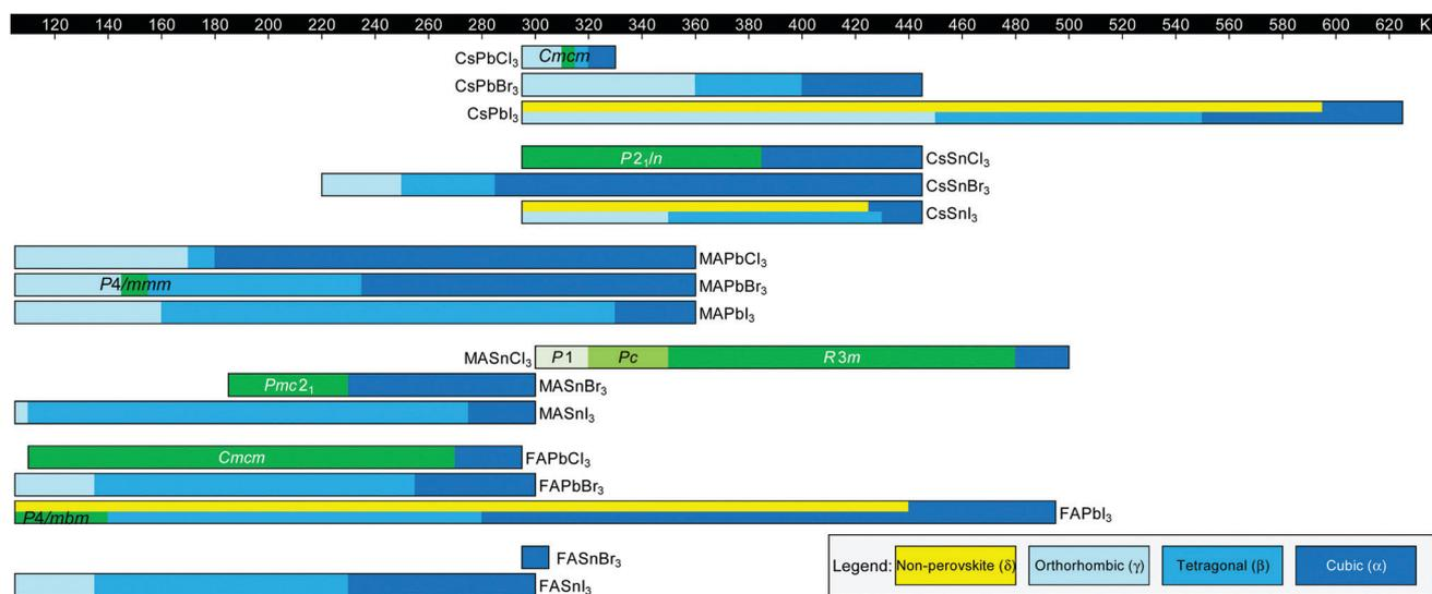
Fig. 3 Summary of phase transition temperatures in halide perovskites reported in the literature collected at ambient pressure as a function of composition.<sup>6,8,20–48</sup> Cubic structures exhibit  $Pm\bar{3}m$  symmetry, tetragonal structures exhibit either  $I4/mcm$  or  $P4/mbm$  symmetry, and the orthorhombic phase exhibits  $Pnma$  symmetry, unless otherwise noted. Green colors indicate phases not represented by the above categories.
