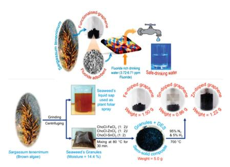
Fig. 13 Deep eutectic solvent-promoted preparation of functionalized graphene nanosheets from seaweed granules for producing safe-drinking water (reproduced from ref. 159 with permission from the American Chemical Society).
