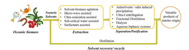
Fig. 8 General scheme for the extraction and purification of renewable chemicals/products from oceanic biomass.
