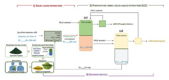
Fig. 6 Schematic of the integrated process for the extraction and purification of chlorophyll a and xanthophylls (reproduced from ref. 122 with permission from the American Chemical Society).
