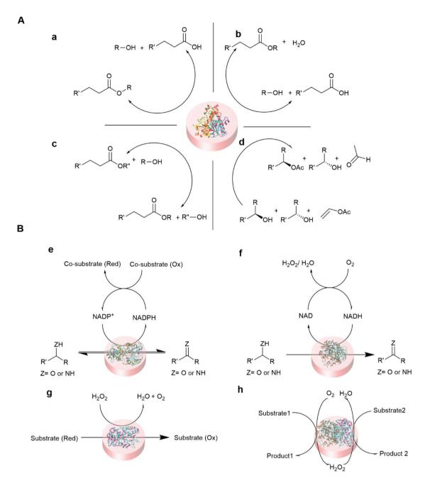
Fig. 5 Representative reaction schemes of immobilized hydrolase and oxidoreductase biocatalysis. (A) Hydrolase (lipase) catalyzed reaction<sup>100,101</sup> (a) hydrolysis (b) esterification (c) transesterification, and (d) kinetic resolution. (B) Oxidoreductase catalyzed reactions<sup>102,103</sup> (e) dehydrogenase (f) oxidase (g) peroxidase and (h) cascade reaction of oxidase and peroxidase.
