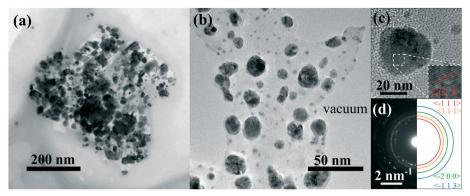
Fig. 5 (a) Bright field TEM image of an agglomeration of well separated nanostructures. (b) Higher magnification of a portion of CuO nanoparticles in the PEC matrix. (c) HR-TEM of a copper oxide nanoparticle. (d) Left: SAED of a portion of the nanoparticle. Right: Sketch of some diffraction rings, the interplanar spacings of which are in agreement with theory.<sup>56</sup>
