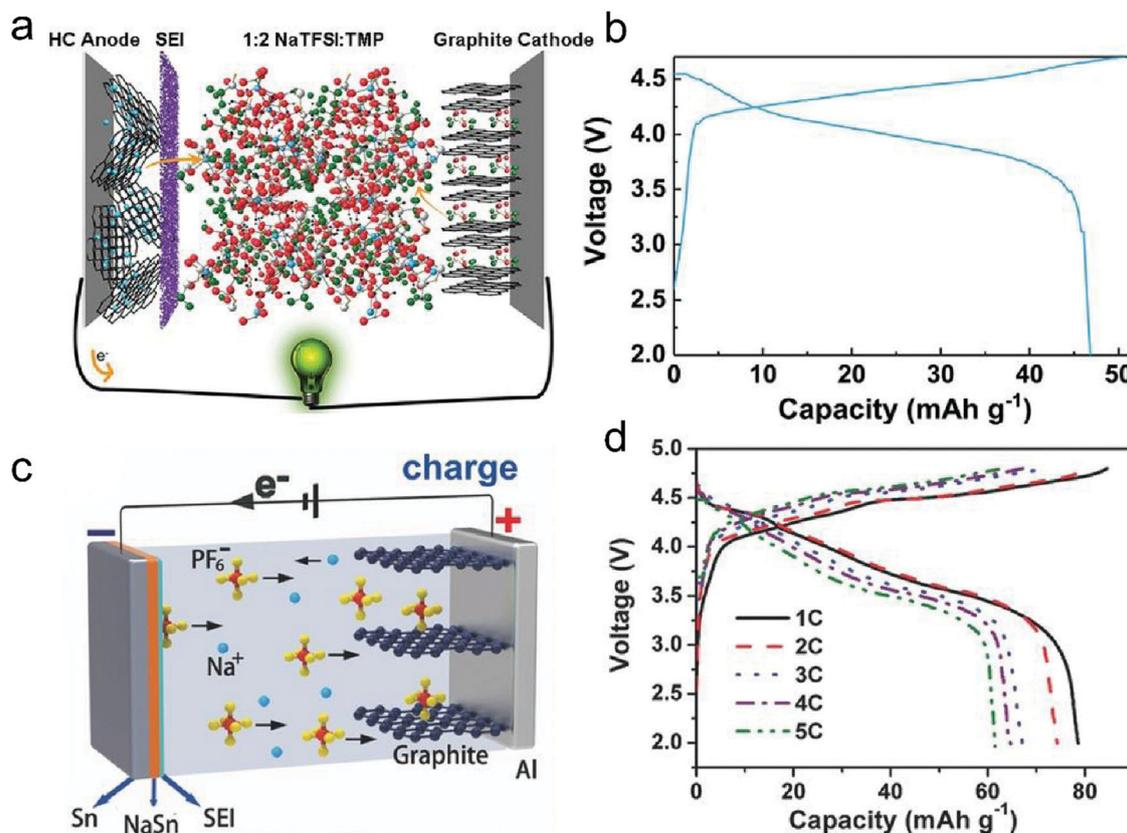
Fig. 27 (a) Schematic illustration and (b) typical charge–discharge curves of Na<sup>+</sup>-dual carbon batteries using a 1 : 2 NaTFSI : TMP electrolyte at 500 mA g<sup>-1</sup>. Reproduced from ref. 397 with permission from Wiley-VCH. (c) Schematic illustration of the working mechanism and (d) charge–discharge curves of a Sn//C DIB at various current rates from 1 to 5C. Reproduced from ref. 197 with permission from Wiley-VCH.
