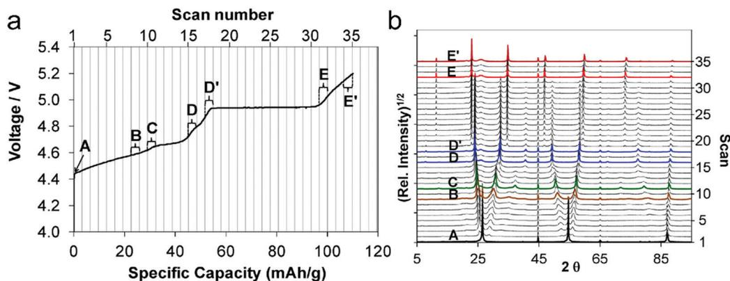
Fig. 9 (a) First charge curve and (b) corresponding *in situ* XRD spectra (5–90°  $2\theta$ ) of the graphite cathode during PF<sub>6</sub><sup>-</sup> intercalation. Reproduced from ref. 129 with permission from American Chemical Society.
