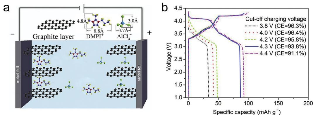
Fig. 32 (a) Operation principle of the DIB containing  $(\text{DMPI}^+)(\text{AlCl}_4^-)$  as an IL electrolyte. (b) Charge/discharge curves of the DIB cell at cut-off charging voltages of 3.8–4.4 V. Reproduced from ref. 439 with permission from Elsevier.
