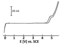
**Fig. 1** Cyclic voltammogram of liquid SO<sub>2</sub> and CsAsF<sub>6</sub> (~4 mM); conditions: Pt working electrode, T = 203 K; SCE = saturated calomel electrode. Figure adopted from Bard (refurbished).<sup>40</sup> Depicted upon permission from John Wiley & Sons.
