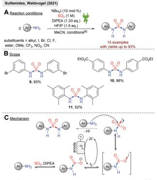
Scheme 2 Electrochemical synthesis of symmetric sulfamides; [a]: Pt electrodes, r.t., 14 h, 7.5 mA cm<sup>-2</sup> (galvanostatic), 2.5 F, divided cell (glass frit).
