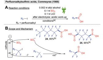
Scheme 7 Electrochemical synthesis of perfluoroalkylsulfinic acids; [a]: DMF/H<sub>2</sub>O (9:1), 20 °C, carbon fiber electrodes, divided cell (glass frit), 1–12 mA cm<sup>-2</sup> (galvanostatic), ~1.05 F; [b]: yield determined by NMR integration (<sup>19</sup>F NMR).
