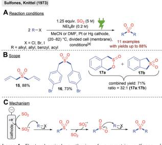
Scheme 4 Electrochemical synthesis of symmetric sulfones; [a]: potentiostatic conditions: -0.7 V vs. Ag/AgCl, 1 F mol<sup>-1</sup> or galvanostatic conditions: 300 mA cm<sup>-2</sup> and 500 mA cm<sup>-2</sup>, 2000–10000 C.
