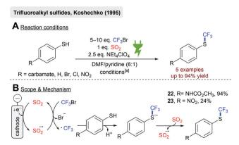
Scheme 6 Electrochemical synthesis of trifluoroalkyl sulfides catalyzed by the SO<sub>2</sub> anion radical; [a]: r.t., Pt||Pt, divided cell (glass frit), -0.9 to -1.0 V (potentiostatic) vs. Ag/AgNO<sub>3</sub>, 0.125–1 F.
