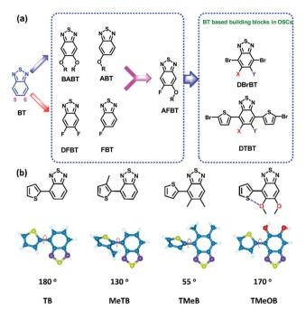
Fig. 1 (a) Evolution of the BT units, and (b) dihedral angles of TB, MeTB TMeTB and TMeOB according to DFT calculations.71
