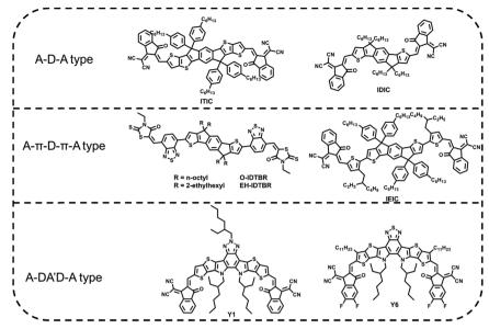
Fig. 6 Typical chemical structures of FREAs.
