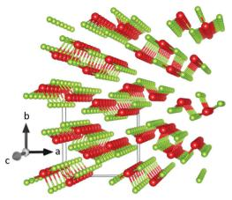
Fig. 1 Sb<sub>2</sub>Se<sub>3</sub> crystal structure drawn in VESTA 3 (ref. 2) – antimony atoms are shown in red and selenium atoms in green. The solid line cuboid represents the unit cell. The axes labels correspond to the Pbnm setting of space group 62.
