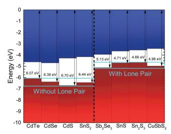
Fig. 7 Ionization potential for  $Sb_2Se_3$  from the photoemission results in Fig. 6, compared with literature values for other materials. 23,24,49,50 The zero of the energy scale corresponds to the vacuum level. The materials are labelled as without or with lones pair 5s<sup>2</sup> electrons.
