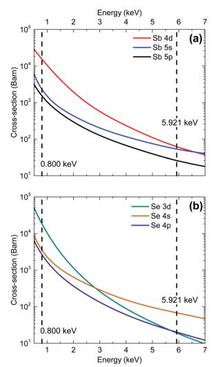
Fig. 2 Photoionization cross-section energy dependence for each valence orbital in (a) antimony and (b) selenium.<sup>25</sup>
