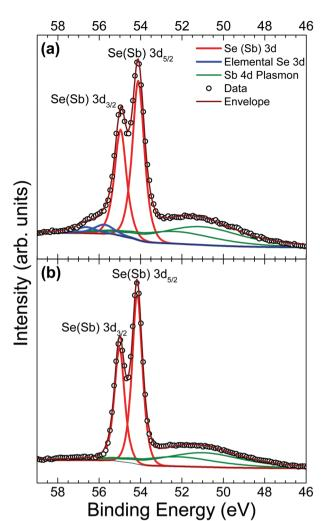
Fig. 4 Se 3d HAXPES data from an Sb<sub>2</sub>Se<sub>3</sub> crystal (a) before and (b) after in situ cleaving.
