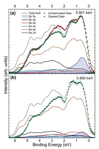
Fig. 5 VB XPS spectra from an Sb<sub>2</sub>Se<sub>3</sub> single crystal sample for (a) hard X-rays with a photon energy of 5.921 keV (HAXPES), before and after in situ crystal cleaving; and (b) soft X-rays with a 0.800 keV photon energy after in situ cleaving. Both are plotted with total and partial theoretical VB DoS calculations.
