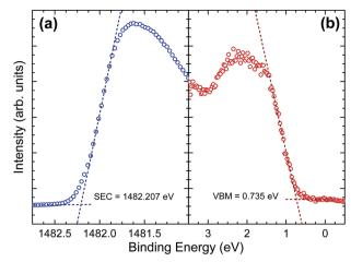
(a) Secondary electron cut-off (blue) and (b) valence band maximum (red) of in situ cleaved Sb<sub>2</sub>Se<sub>3</sub> bulk crystals with straight line fits used to determine the binding energy of the cut-offs. The incident photon energy is 1486.6 eV.
