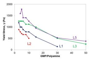
Fig. 5 Plot of the yield stress as a function of the GMP/polyamine auotient
