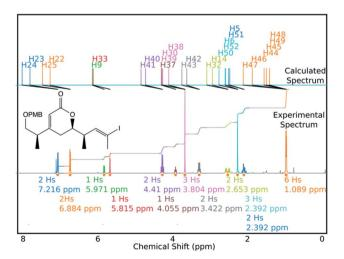
Fig. 9 DP4-AI processed and assigned <sup>1</sup>H spectrum of molecule BYH1 (taken in chloroform).
