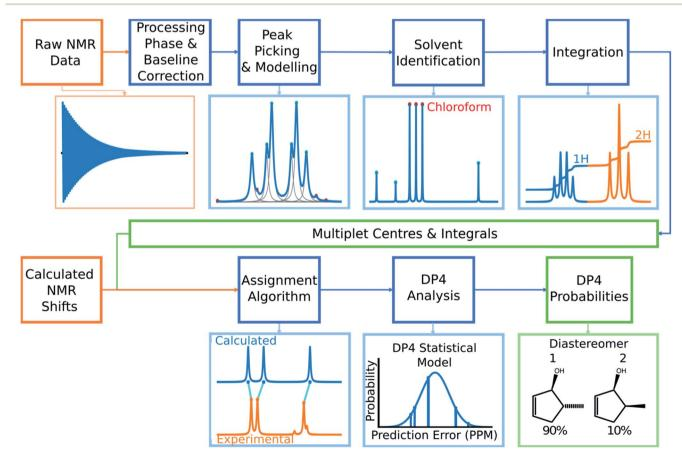
Fig. 2 The overall structure of DP4-Al. Raw NMR data is processed in a series of stages to yield experimental multiplet shift values and their integrals. The program then takes shifts calculated using DFT for each atom in the molecule and assigns them to the experimental peaks. This assignment is then used to calculate a DP4 probability for each diastereomer.
