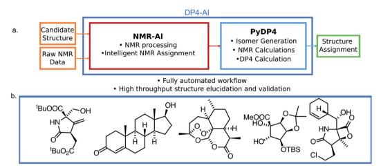
Fig. 1 (a) The structure of DP4-AI. This system affords fully automated stereochemistry elucidation, only the raw NMR data is a required input from the user. (b) Example structures with stereochemistry correctly predicted fully automatically using DP4-AI integrated in PyDP4.
