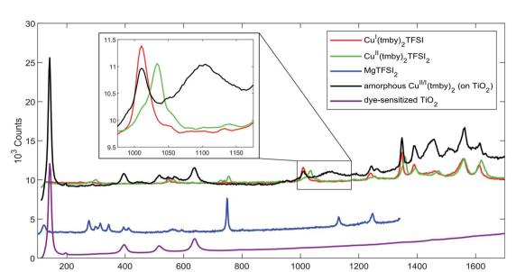
Fig. 4 Raman spectra of  $Cu^{II/I}(tmby)_2$  TFSI<sub>(2)</sub> and MgTFSI<sub>2</sub> (powders), DSCs sensitized with the XY1:L1 sensitizer combination as well as (sensitized) DSCs containing amorphous  $Cu^{II/I}(tmby)_2$  TFSI<sub>(2)</sub> hole transport material. The two latter spectra were recorded inside the 'sandwich' DSC. Spectra are offset for clarity.
