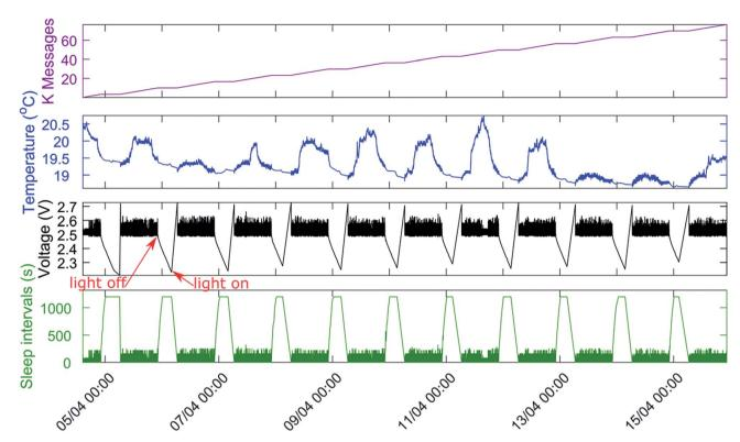
Fig. 6 Atmega328P-based wireless node equipped with transceiver and AVX 6.0 V 0.47 F supercapacitor. The sensor is powered by five serial 3.2 cm<sup>2</sup> photovoltaic cells (total 16.0 cm<sup>2</sup>). The sensor was tested in simulated light intervals of 16 hours "day" (1000 lux) and 8 hours darkness (10 pm-6 am, red arrows).
