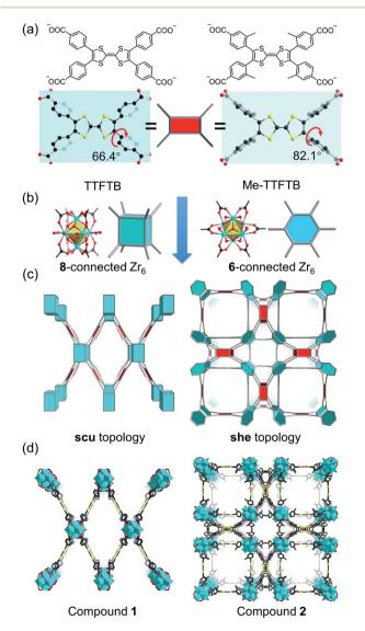
Fig. 1 Topologically guided steric tuning strategy for MOF design (a) TTFTB and Me-TTFTB linkers with different conformations. (b) 8-connected and 6-connected  $Zr_6$  clusters. (c) Targeted topologies formed by  $Zr_6$  clusters and conformationally differing linkers. (d) Crystal structures of compounds 1 and 2. Color scheme: Zr, cyan; Zr0, red; Zr1, Zr2, Zr3, Zr4, Zr5, Zr6, Zr7, Zr7, Zr8, Zr8, Zr9, Z
