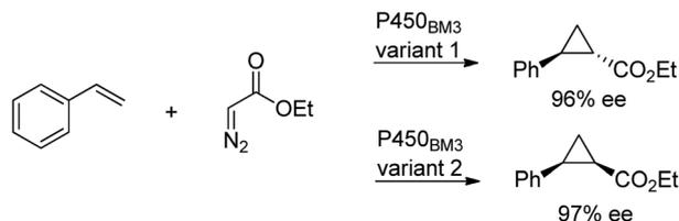
Scheme 22 Stereoselective cyclopropanation reaction of P450<sub>BM3</sub>.
