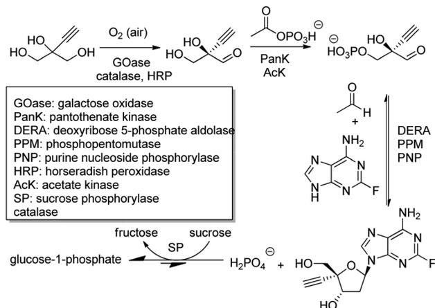
Scheme 21 Biocatalytic cascade synthetic route to islatravir.
