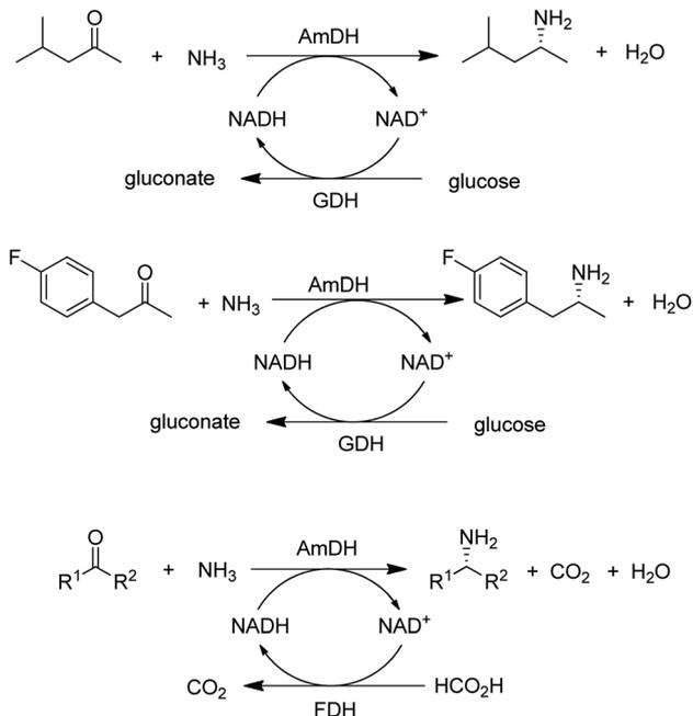
Scheme 6 Enzymatic primary amine synthesis with amine dehydrogenases.
