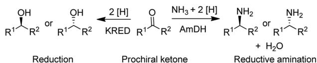
Scheme 3 Reduction and reductive amination of ketones.
