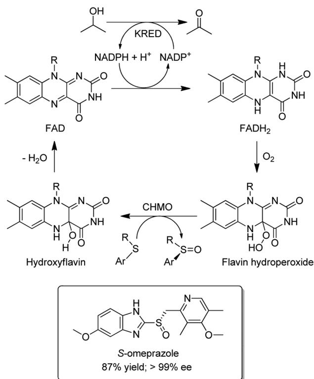
Scheme 14 Enantioselective sulfoxidation using an ADH/BVMO cascade.
