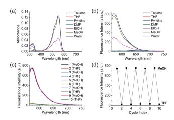
Fig. 1 (a) Absorption spectra and (b) fluorescence spectra of Dye1 in various polar and non-polar solvents. (c) Fluorescence spectrum and (d) fluorescence intensities of Dye1 with the polarity of MeOH and THF solvents reversed for five cycles. All concentrations for the spectral measurements were 1 µM, the excitation wavelength was 552 nm, and the fluorescence intensity was acquired at 573 nm.
