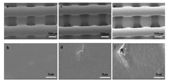
Fig. 1 SEM images: PCL scaffold at 300  $\mu$ m (a), PCL scaffold at 5  $\mu$ m (b), PCL/HA scaffold at 300  $\mu$ m (c), PCL/HA scaffold at 5  $\mu$ m (d), EPL/PCL/HA scaffold at 300  $\mu$ m (e), EPL/PCL/HA scaffold at 5  $\mu$ m (f).
