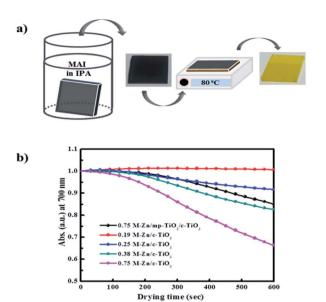
Fig. 3 (a) The decomposition behaviors and (b) the decrease in the absorbance at 700 nm over 600 s of the MAPbl<sub>3</sub> perovskite film fabricated by this sequential dip-coating deposition on ZnO/c-TiO<sub>2</sub> layer observed during solvent drying.
