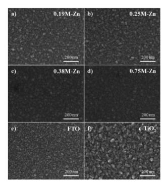
Fig. 2 SEM surface topologies of thin ZnO layers fabricated from ZnO sol-gel precursors prepared with various Zn concentrations of (a) 0.19 M-Zn, (b) 0.25 M-Zn, (c) 0.38 M-Zn, and (d) 0.75 M-Zn over the c-TiO<sub>2</sub> layer, which were compared to those of the (e) bare FTO substrate and (f) c-TiO<sub>2</sub> layer deposited on the FTO.
