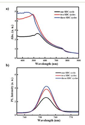
Fig. 5 (a) UV-vis absorption and (b) photoluminescence spectra for these PHJ MAPbl $_3$  perovskite films deposited on ZnO (0.25 M- Zn)/c-TiO $_2$ /FTO under designed SDC cycles.
