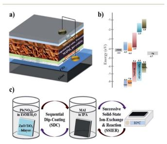
Fig. 1 Description of (a) PHJ PrSC structure, (b) energy level diagram, and (c) the preparation of the MAPbI $_3$  perovskite films by sequentially dip-coating a ZnO-covered c-TiO $_2$ /FTO substrate in aqueous Pb(NO $_3$ ) $_2$  and MAI solutions.
