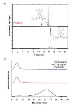
Fig. 2 (A) HPLC and radio-HPLC traces for complexes 3 (blue), and [68Ga]-3 (red). (B) Radiochemical data for the [68Ga]-radiolabelling of GO nanocomposites. Small impurities at 11 min are assignable to protonation and/or Ga-Cl/Ga-OH exchanges in water. Radio-iTLC of [68Ga] Ga@GO and [68Ga]Ga-2@GO (C18 paper TLC, mobile phase: 0.35 M EDTA).
