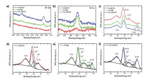
Fig. 6 XPS spectra of core levels (a) Zn 2p, (b) N 1s, (c) Ga 3d. (d) Ga 3d energy region for the Ga@GO sample with a fit of a Ga<sup>3+</sup>, 3 Ga-O singlet, Ga<sup>1+</sup>, and Ga-Cl, (e) and (f) same scenario than (d) but for the Ga (3) and Ga-2@GO samples.
