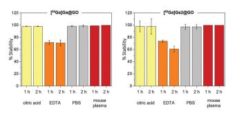
Fig. 3 Kinetic stability tests: [68Ga]Ga@GO (left) and [68Ga]Ga-2@GO (right) Nanocomposites were exposed up to 2 h to challenges under various incubation conditions described in ESI.† Error bar stands for standard error (±SE), calculated from three independent, repeated, measurements.
