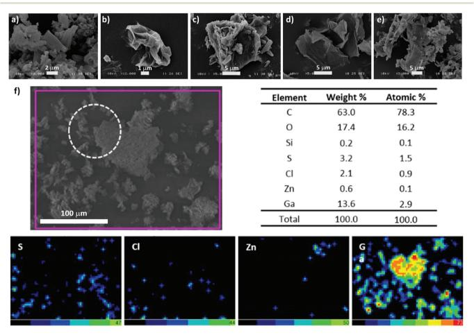
Fig. 5 Scanning Electron Microscopy (SEM): micrographs and corresponding EDX analysis of complexes and nanocomposites. (a) Complex 2; (b) GO; (c) 2@GO; (d) Ga@GO and (e) Ga-2@GO. Scale bars: (a) 2 µm, (b) 1 µm, (c), (d) and (e) 5 µm. (f) SEM image and corresponding EDX elemental analysis and EDX mapping image (S, Cl, Zn, Ga) of Ga-2@GO nanocomposite.
