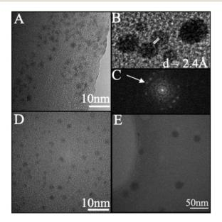
Fig. 2 Representative TEM image of (A) undoped CDs, 4 h reaction time (diameter =  $2.5 \pm 0.3$  nm). (B) Undoped CDs, 4 h reaction time exhibiting lattice. (C) FFT of (B) with spots matching lattice fringes at a *d*-spacing of 2.40 Å. (D) 1 : 2 NCD, 4 h (3.0  $\pm$  0.5 nm). (E) Undoped CD, 24 h (diameter =  $16 \pm 2$  nm). All experiments were performed at room temperature under 200 keV acceleration voltage and images were processed using ImageJ
