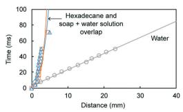
Higher surface tension leads to longer distance traveled with higher speed
