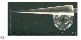
Fig. 15 (a) Effect of cone wettability on air bubble movement (adapted from ref. 18). The distance traveled by air bubbles is shown as a function of time. (b) Optical images of air bubbles at deposition and at equilibrium on cones with various wettabilities (adapted from ref. 18).
