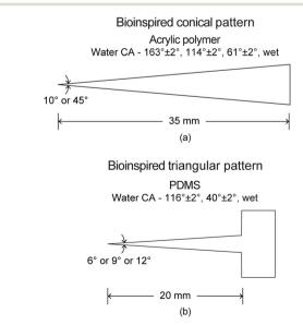
Fig. 10 Schematic of bioinspired (a) conical surface and (b) triangular pattern with a reservoir with various wettabilities (adapted from ref. 17 and 18).
