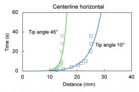
Smaller tip angle results in longer distance traveled and faster speed
