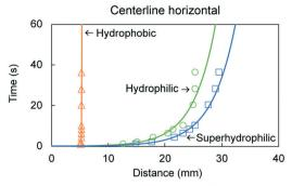
High wettability results in longer distance traveled at larger speed. A bubble on hydrophobic surface does not moves.
