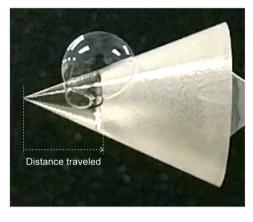
Fig. 14 (a) Effect of cone tip angle on the air bubble movement (adapted from ref. 18). The distance traveled by the air bubble is shown as a function of time. (b) Optical images of air bubbles at deposition and at equilibrium on the cone with tip angle 45° (adapted from ref. 18).
