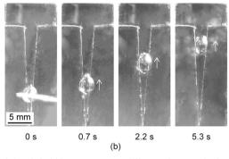
Fig. 16 (a) Selected photographs (top view) of the air bubbles transport at different times on hydrophilic and superhydrophilic triangular patterns with various wettabilities (adapted from ref. 17). (b) Air bubble climbs up a vertical superhydrophilic triangular pattern (adapted from ref. 17). Arrows shown represent air bubbles movement observed in videos
