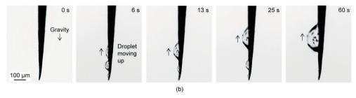
Fig. 2 (a) Mechanism used by cactus to move water droplets (adapted from ref. 25). (b) Optical images of water droplets initially collected at the barb tip and/or spines of Ferocactus latispinus, climbed up over the cactus spine due to Laplace pressure gradient (adapted from ref. 25). Droplets defy gravity.
