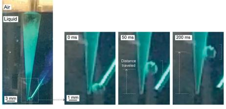
Fig. 24 Optical images of underwater air bubbles traveling on cones under various liquids (adapted from ref. 19).
