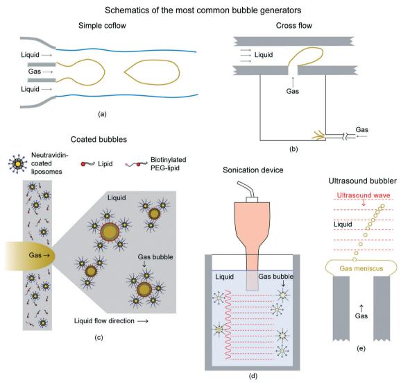
Fig. 7 Schematics of the most common bubble generators.<sup>35</sup> (a) Simple coflow configuration in which gas and liquid flow in the same direction. (b) Cross flow configuration in which the gas injected perpendicular to the liquid stream. (c) Creating shell for gas bubbles (d) sonicator inducing the growth and collapse of bubbles by means of an ultrasound field. (e) Ultrasound wave-driven generation of a train of monodisperse gas bubbles from a meniscus attached to the gas injector.
