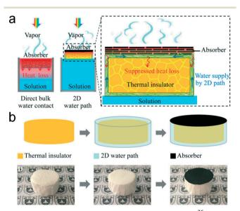
Fig. 4 Typical evaporator in indirect contact mode. 36 (a) The comparison and the mechanism of the interfacial solar evaporator. The heat loss is strongly suppressed by the insulator, and water can be continuously pumped to the evaporating interface through the 2D path. (b) The rapid fabrication of the evaporator in indirect contact mode.
