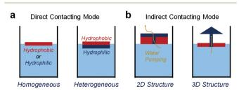
Fig. 2 The classification of current solar evaporators. (a) Direct contact mode with homogeneous or heterogeneous structures. (b) Indirect contact mode with 2D or 3D hierarchical structures.
