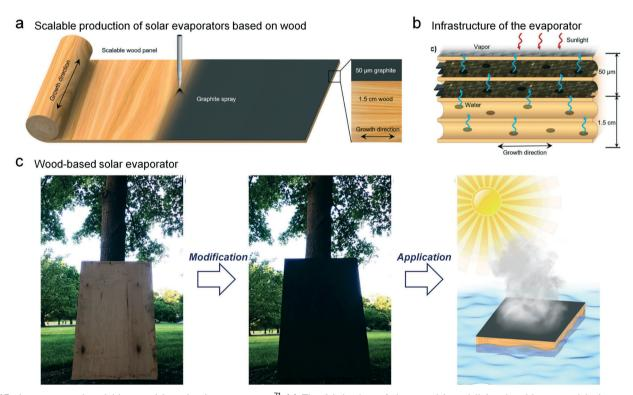
Fig. 13 Low-cost and scalable wood-based solar evaporator. 71 (a) The fabrication of the wood-based light-absorbing material via a graphite spraying method. The thickness of the light-absorbing layer is 50 µm and that of the insulating layer is about 1.5 cm. (b) The water can transfer to the evaporation interface through the wood lumens. (c) The demonstration of scalable fabrication and the application of the wood-based floatable evaporator.
