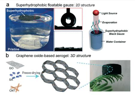
Fig. 5 Intrinsically floatable solar evaporators. (a) The carbon black-based, self-cleaning, superhydrophobic gauze for efficient solar evaporation at the air-water interface.<sup>45</sup> (b) The graphene oxide-based aerogel with ultralow density for solar steam generation.<sup>47</sup>
