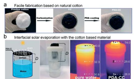
Fig. 12 Low-cost cotton based solar evaporator. (a) The rapid fabrication of light absorbing cotton. (b) The oil lamp inspired solar evaporator exhibits an obvious interfacial heating ability.<sup>70</sup>
