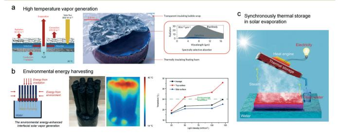
Fig. 10 Innovative solar evaporators with heat managing design. (a) The evaporator with multi-level high insulation for high temperature vapor generation.<sup>59</sup> (b) Smart design for harvesting environmental energy through a wetted side wall. (c) Harnessing the heat of vapor by the water collector for electricity generation.66
