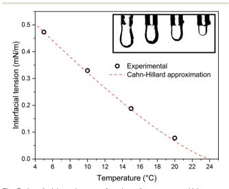
Fig. 3 Interfacial tension as a function of temperature. Values were determined via pendant drop experiments of 5CB-rich droplets immersed in a MeOH-rich phase. Representative droplets are shown in upper right box, from left to right at 5 °C, 10 °C, 15 °C and 20 °C.
