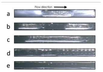
Fig. 4 Temperature-induced tuning of different flow patterns. Observed flow patterns at a fixed flow rate (70  $\mu l \ min^{-1}$ ) and channel cross section (700  $\times$  700  $\mu m^2$ ) with temperature as the only experimental variable: a) -1 °C, b) 5 °C, c) 10 °C, d) 15 °C and e) 20 °C. black arrow indicates flow direction.
