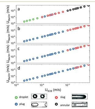
Fig. 2 Estimated velocity of each phase after phase separation and corresponding two-phase regime. Four different regimes were observed, namely droplet, plug, slug and annular flow. a) 20 °C, b) 15 °C, c) 10 °C and d) 5 °C.
