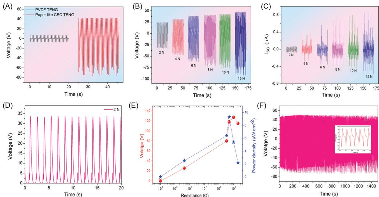
**Fig. 5** (A) Relative output voltage of the PVDF and P-CEC-based TENG, (B and C) output voltage and current of the P-CEC TENG as a function of applied compressive force, respectively, (D) rectified voltage of the P-CEC TENG at a constant applied compressive force of 2 N, (E) output voltage and maximum peak power of the P-CEC TENG as a function of load resistance, and (F) endurance test of the P-CEC TENG over 1500 s at a constant applied force.
