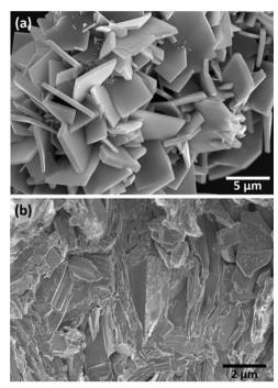
Fig. 6 SEM micrograph of  $Sn_{1-\delta}S$ : (a) powder synthesized by the microwave-hydrothermal method and (b) the cross-section of the SPS sintered pellet.
