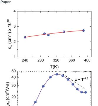
Fig. 8 (a) Temperature dependence of the Hall carrier concentration  $(n_{\rm H})$ . (b) Temperature dependence of the Hall carrier mobility  $(\mu_{\rm H})$  of  ${\rm Sn}_{1-\delta}{\rm S}$ . The Hall carrier density of  $\sim 2.5\times 10^{18}~{\rm cm}^{-3}$  measured at room temperature is assumed to be unchanged up to 823 K. The solid lines are a guide to the eye. The dotted line corresponds to the  $\mu\sim T^{-1.5}$  temperature dependence.
