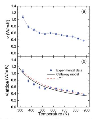
Fig. 10 Temperature dependence of the (a) total thermal conductivity and (b) lattice thermal conductivity of microwave-synthesized  $\mathrm{Sn}_{1-\delta}\mathrm{S}$ . The black solid line represents the data calculated using the Callaway model, <sup>76</sup> while the dotted line shows the  $\sim \mathcal{T}^{-1}$  fit.
