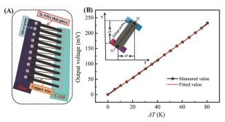
Fig. 6 The as-assembled TEG prototype with 10 pieces of the optimized Te NWs thin pieces (A). The output voltage of the TEG versus the temperature difference (B). The inset is the schematic illustration for measuring the S value.
