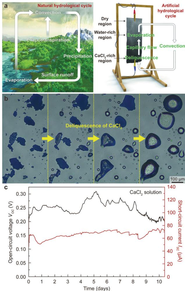
**Fig. 2** Artificial hydrological cycle system for the STEPG. (a) Schematic illustration of natural hydrological cycle and artificial hydrological cycle for the STEPG. (b) Optical microscope image of CaCl<sub>2</sub> exposed to 40% RH, showing typical deliquescent behavior. (c) Continuous  $V_{oc}$  and  $I_{sc}$  generated by applying 0.25 mL of saturated CaCl<sub>2</sub> solution onto a stacked carbon black-coated cotton fabric (base resistance: 5 kΩ) at 25 °C and 35% RH.
