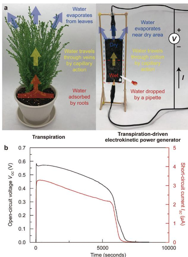
**Fig. 1** TEPG. (a) Transpiration of plants (left) and the electrokinetic power generator whose operation resembles the transpiration of plants (right). (b) Measured  $V_{OC}$  and  $I_{SC}$  from the 120 k $\Omega$  TEPG generated by dropping 0.25 mL of DI water.
