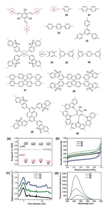
Fig. 9 Chemical structures of polymers 30-40. (a) HOMO and LUMO band positions of polymers 30-33. (b) Nitrogen sorption isotherms, (c) photoluminescence spectra, and (d) hydrogen evolution of polymers 34-36. Reprinted with permission from ref. 112 and 113. Copyright 2017 Wiley-VCH and 2016 American Chemical Society.
