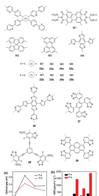
Fig. 8 Chemical structures of D-A type CPPs and (a) the optical gaps as well as (b) photocatalytic H2 production of polymers 22-25 (P-a: 22a-25a; P-b: 22b-25b). Reprinted with permission from ref. 105. Copyright 2016 American Chemical Society.
