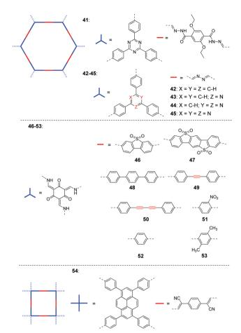
Fig. 10 Chemical structures of COFs 41–54 for photocatalytic H<sub>2</sub> production under visible light.
