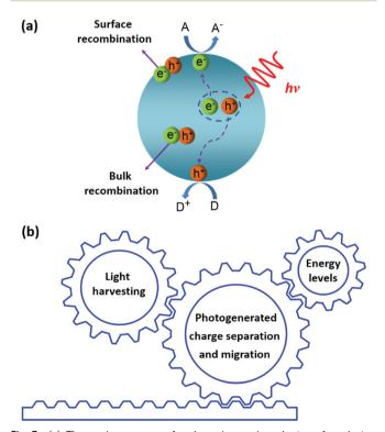
(a) The main process of polymeric semiconductors for photo-Fia. 3 catalysis (D: electron donor; A: electron acceptor) and (b) critical factors affecting their photocatalytic performances
