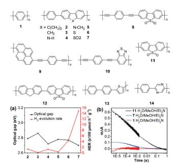
Fig. 5 Chemical structures of polymers 1-14, (a) the correlation between the photocatalytic  $H_2$  evolution and their optical gaps of polymers 2–7 (>420 nm); (b) transient kinetics probed at 630 nm for polymers 1, 7, and 11 in the Et<sub>3</sub>N/CH<sub>3</sub>OH/H<sub>2</sub>O mixture (excited at 355 nm). Reprinted with permission from ref. 72. Copyright 2018 Nature Publishing Group.
