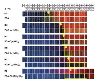
Fig. 11 Photographs of the alkly-diamine-intercalated PDA samples with changes of the temperature by the protocol including heating (the upper panels) and subsequent cooling (the lower panels) as shown in the top part. The yellow arrows indicate the color-change temperature to red recognized by the naked eye. The yellow frames in the lower panels show the reversible color change to the original blue. Reprinted with permission from Springer Nature.83
