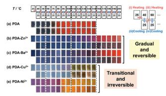
**Fig. 9** Photographs of PDA and PDA-M<sup>2+</sup> with changes of the temperature by the protocol including heating (the upper panels) and subsequent cooling (the lower panels) as shown in the top part. (a) PDA, (b) PDA-Zn<sup>2+</sup>, (c) PDA-Ba<sup>2+</sup>, (d) PDA-Cu<sup>2+</sup>, and (e) PDA-Ni<sup>2+</sup>. The temperature of the samples in the panels (a)–(e) is referred to the same position in the top part. Reprinted with permission from Wiley-VCH.<sup>79</sup>
