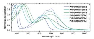
Fig. 1 Normalized UV-vis absorption spectra of **PNDI(MBS)2T-6T** in CB  $(0.1~{\rm g~L^{-1}})$  and as annealed films.
