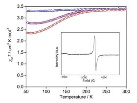
Fig. 5  $\chi_{\rm M}T$  vs. T plot of [FeL<sub>a</sub>(py<sub>2</sub>TTF)]<sub>n</sub> (red) and doped with iodine for 2 days (purple) and 2 weeks (blue). Inset: EPR spectrum of [FeLa(py2TTF)]<sub>n</sub> infused with iodine for 2 weeks showing an oxidised TTF signal.
