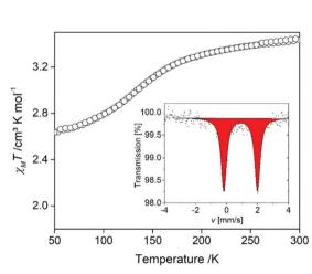
Fig. 4  $\chi_{M}T$  vs. T plot of  $[FeL_a(py_2TTF)]_n$  over the range 300–50–300 K. Inset: Mössbauer spectra at room temperature.
