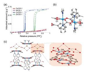
Fig. 2 (a) Adsorption and desorption isotherms for water at 298 K. Filled and open symbols correspond to adsorption and desorption, respectively. Coordination structure of CuCID-1⊃H<sub>2</sub>O around (b) metal ion and (c) O4<sub>w</sub>.
