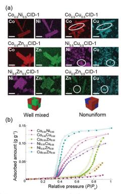
Fig. 4 (a) SEM-EDX maps for M1<sub>0.5</sub>M2<sub>0.5</sub>CID-1. White circles indicate nonuniform areas. Scale bars: 30 µm. (b) Water-sorption isotherms of M1<sub>0.5</sub>M2<sub>0.5</sub>CID-1 at 298 K. Filled and open symbols correspond to adsorption and desorption, respectively.
