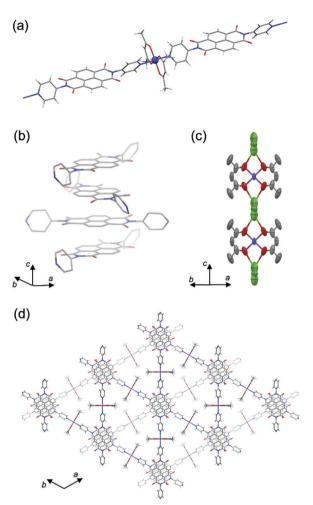
Fig. 1 Crystal structure of PMC-2. (a) One-dimensional coordination polymer in **PMC-2**. (b)  $\pi$ -Stacked NDI column along the c axis. (c) Thermal ellipsoid plot for the [Co(acac)<sub>2</sub>] moieties and Rb<sup>+</sup> ions, which are disordered in three different positions with a total occupancy of 50%. (d) Perspective view of **PMC-2** along the c axis. Hydrogen atoms are omitted for clarity in (b and c). Green, Rb; purple, Co; red, O; blue, N; gray, C; white, H.
