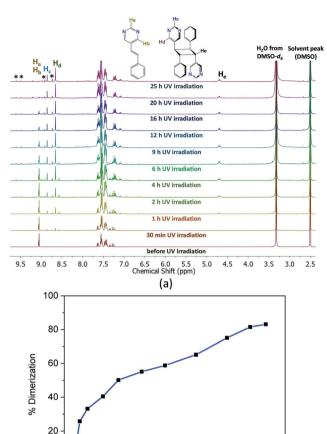
Fig. 2 (a)  $^1\text{H-NMR}$  spectra of **1** (30 min grinding) in DMSO- $d_6$  plotted at different times of UV irradiation. Complete absence of the H<sub>a</sub>, H<sub>b</sub> protons may indicate quantitative consumption of the 5-Spym ligand. However, some unidentified peaks indicate only 83% of *rcct*-bpcb photoproduct formed. (b) Time-dimerization plot for 30 min ground sample shows the progress of the photoreaction under UV light with time.
