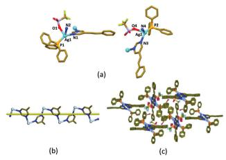
Fig. 1 (a) Coordination geometry around Ag(i) atoms with selected labelling of atoms. (b) A helical polymer strand. (c) Packing of  $\bf 1$  showing different orientations of the 5-Spym arms in the helical one-dimensional CP when viewed from b-axis. The disorder and H-atoms are omitted for clarity.
