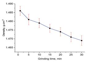
A plot of measured densities of the ground samples with grinding time.
